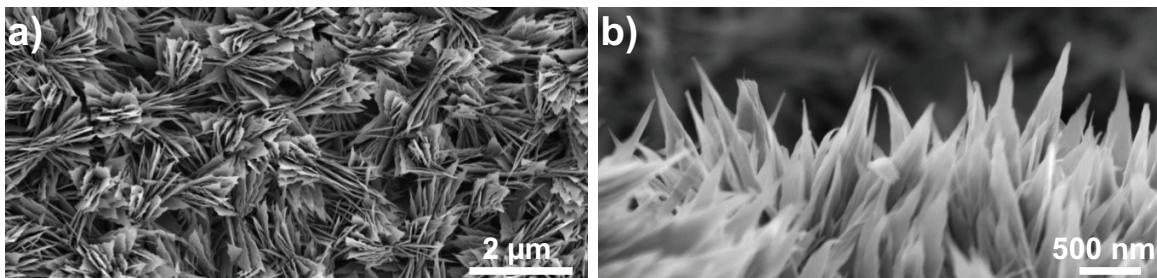
**FIG 1.** Field emission scanning electron microscopy images of a nanostructured copper oxide (CuO) surface with (a) top view, (b) side view. The sharp, knife-like CuO structures have characteristic heights,  $h \approx 1 \mu\text{m}$ , solid fraction,  $\varphi \approx 0.023$ , and roughness factor,  $r \approx 10$ .
